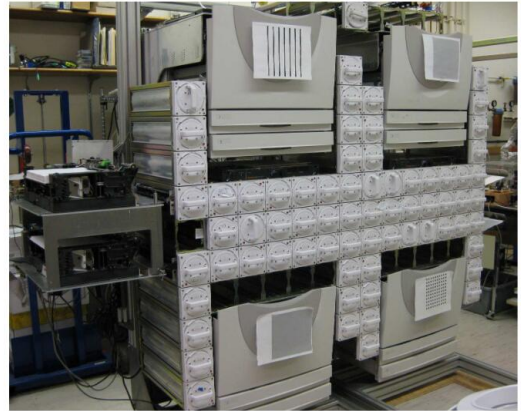
Figure 1: A prototype modular printer built at PARC. The system is composed of approximately 170 individually controlled modules, including four print engines.
